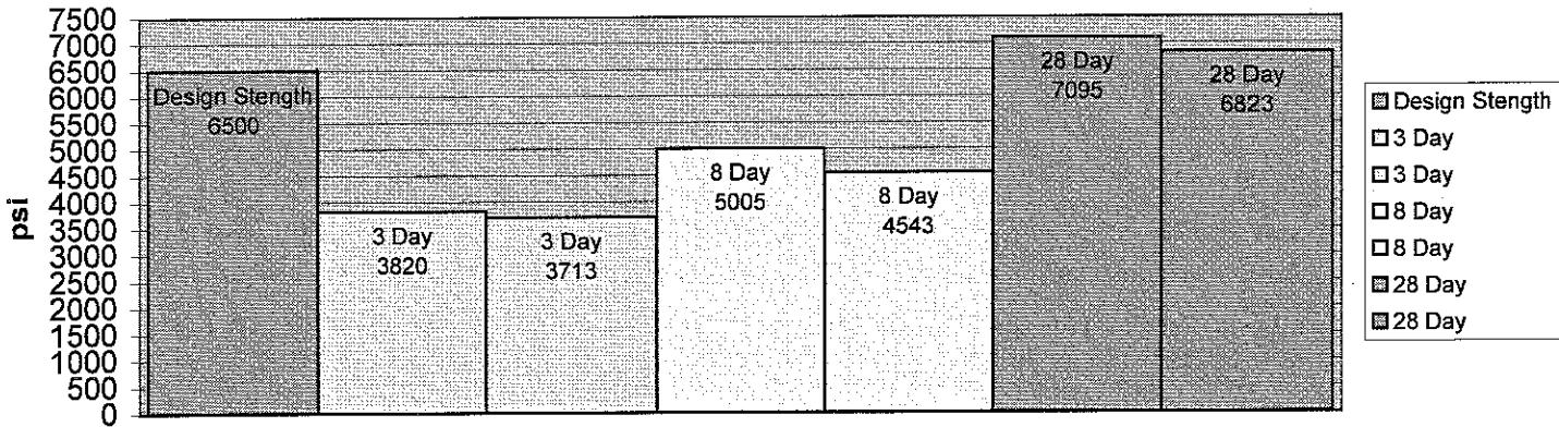
\*Standards state the the specimen should obtain 50% of the design strength by 3 days
